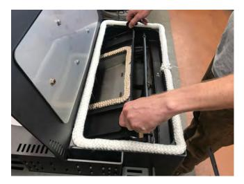
7. Place the sled on a work surface and remove the existing gasket and adhesive. Use a wire brush and vacuum to remove any residual debris.
